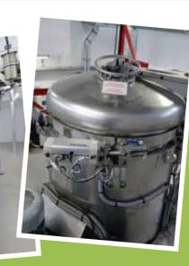
T700 - Maximum process volume capacity 780 L per cycle.
